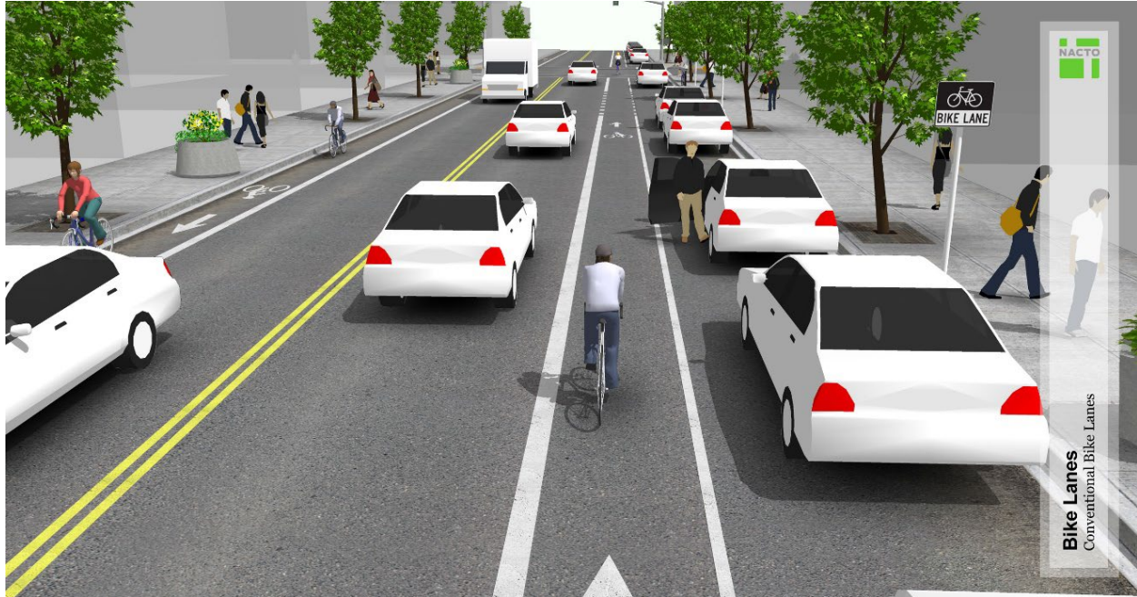
Figure 5-3. Class II bikeway located to the left of the parking lane adjacent to vehicle traffic
