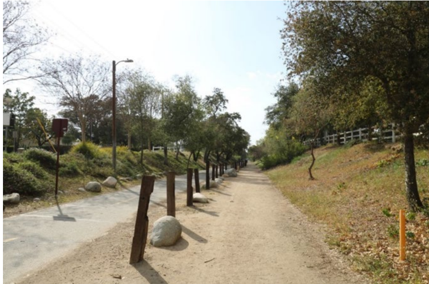
Figure 3-3. Equestrian facilities (right side) should be separated from pedestrian paths and bikeways
